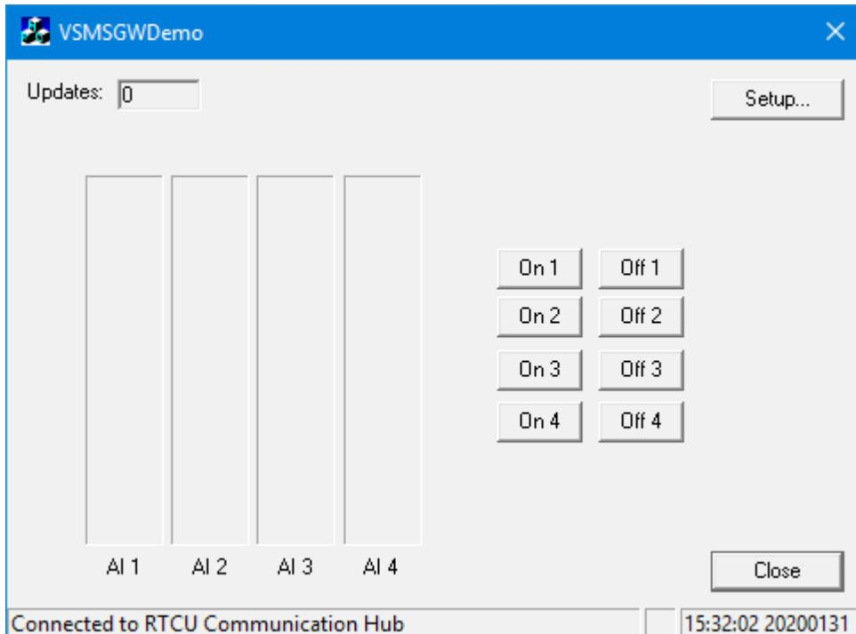
The field “Updates” shows how many messages that has been sent from the device, and the 4 bar graphs shows graphically the values of the 4 analog inputs. By pressing one of the 8 buttons (On 1...4 and Off 1...4) it is possible to control the 4 digital outputs on the RTCU device.
