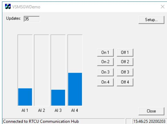
The demo project consists of a PC application and a RTCU application (see Appendix A). The RTCU application sends periodically the values of its 4 analog inputs to the PC application, and the PC application can send commands to the RTCU device that will command one of the four outputs on the RTCU device to switch either on or off.
