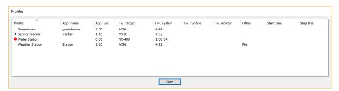
When a new version of the firmware or application is available, edit the profile, and those devices that are affected by the change start the transfer.
