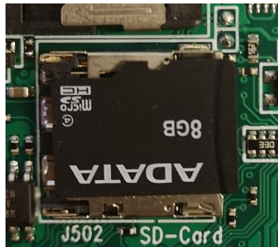
Micro SD card orientation
